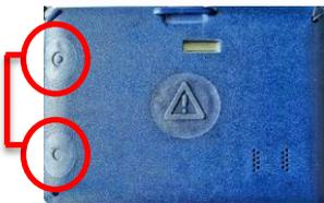
Press and hold the highlighted buttons simultaneously until you feel a vibration. When it switches on, you will feel one vibration and the Identicom will then go through a symbol, light, vibrate and tone sequence.
