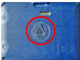
A red alert can be activated by pressing the large round shaped button at the back of the device, or by pulling the Alarm Peg out of the top left corner of the device. It must be used when you require assistance. The red alert button should be pressed for one and a half seconds. The device will give three short burst of vibration to confirm
