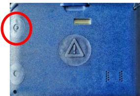
Before carrying out lone working activities you should check your device battery level and phone signal strength by pressing and holding the top left oval shaped button until the LED's start to flash red. After a short while, the battery and signal strength will stop flashing and indicate using the traffic light system: **Green - Good, Amber - Low, Red - Poor battery or signal strength.**
